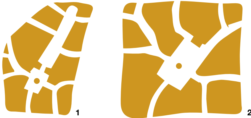
1. Dynamic formal space – length should be limited to avoid monotony for the pedestrian 2. Static formal space in matrix of informal layout
