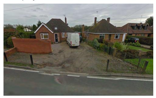
This property has a 1.8m wall set back approximately 4 to 5 meters from the carriageway, and a further railing set back 0.2m from the carriageway. There is a small wall between the railings and the larger brick wall, which it would not be possible to negotiate with a push chair or wheel chair without entering the carriageway.
