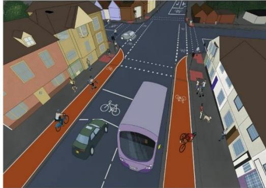
13. We propose to alter the junction with Rosebery Avenue/Guildford Road to make it easier for cyclists to navigate the junction. This includes the introduction of cycle lanes across the junction and new signals programmed to give cyclists more time to cross the junction ahead of traffic. Traffic modelling indicates these changes will not increase congestion at the junction. To what extent do you support these measures?
