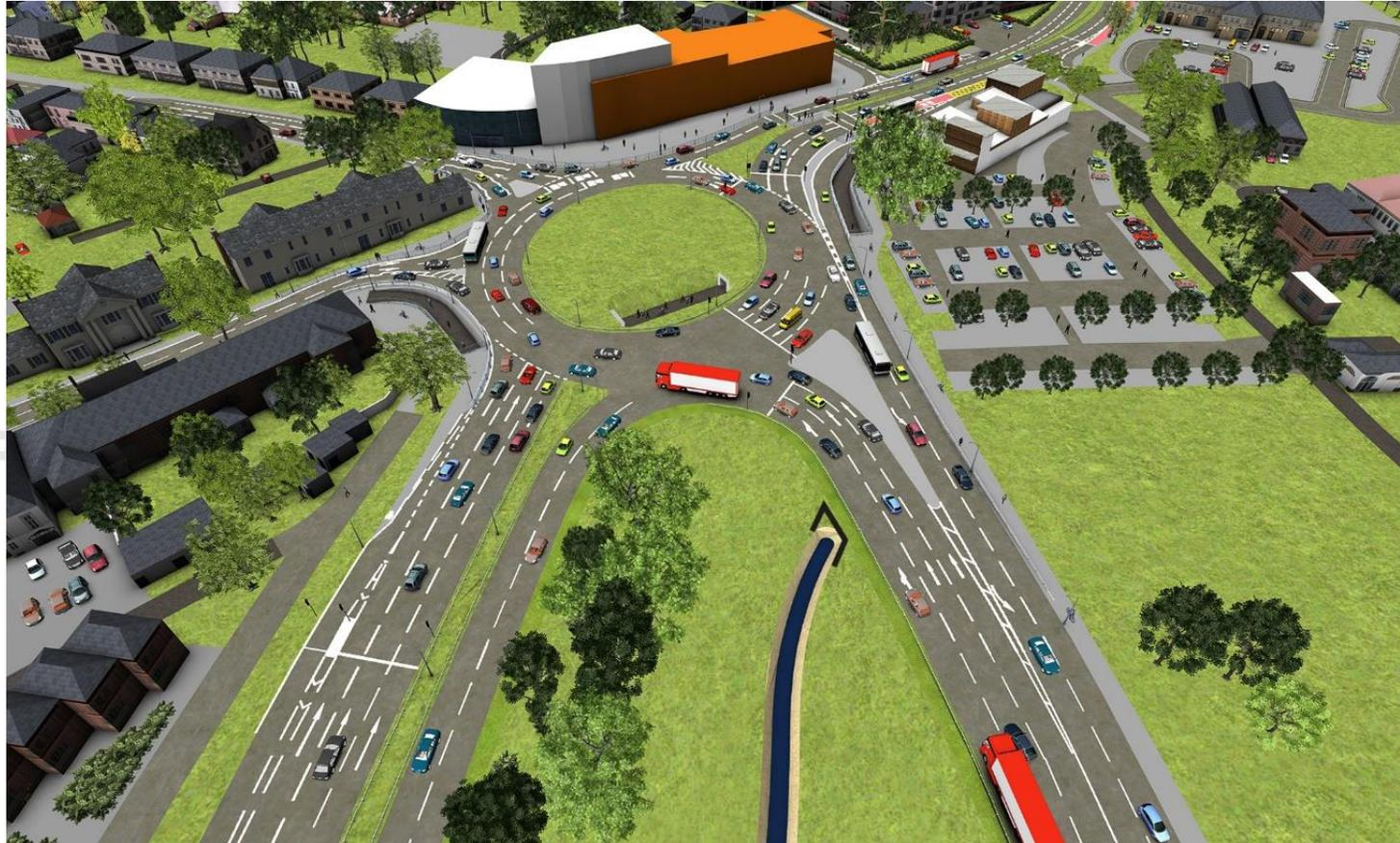
A package of minor highways improvements, including an extension to the Parkway to Chelmer Road slip road, an additional lane on the roundabout between Parkway and Essex Yeomanry Way, an extra lane on entry to the roundabout from Essex Yeomanry Way, bus lanes on either side of Parkway and enhanced pedestrian and cycling routes.
