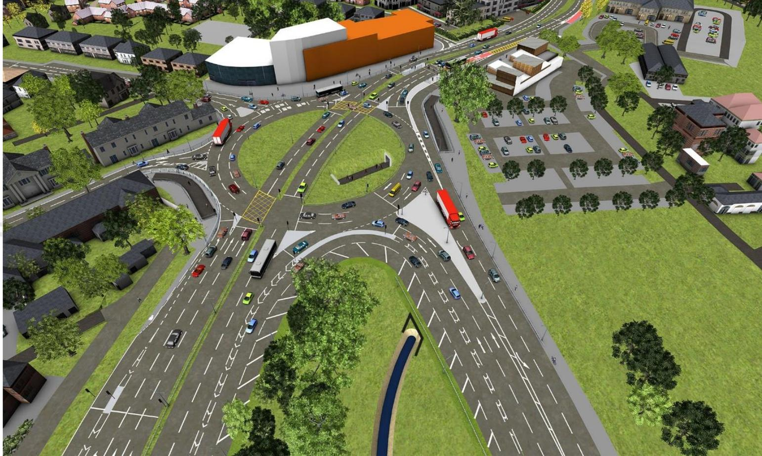
Otherwise known as a throughabout, traffic would be able to travel straight between Essex Yeomanry Way and Parkway through the centre of the junction without using the roundabout. Traffic travelling to other arms of the junction would use the roundabout. Traffic signals would be used to manage traffic flows and priority.
