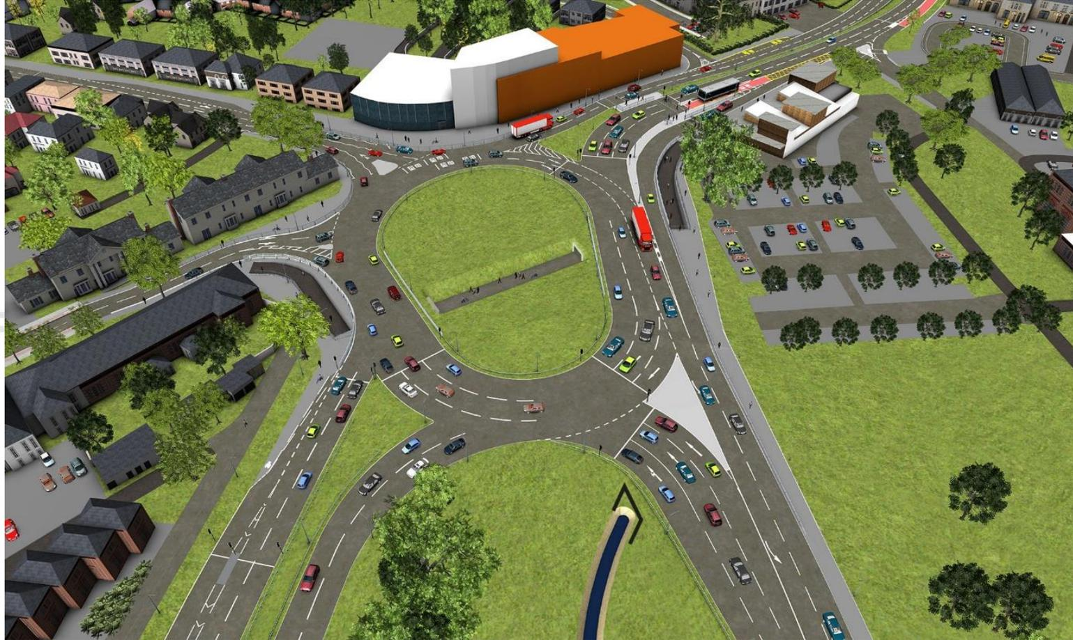
The existing roundabout would be enlarged into the floodplain, creating a larger circulatory. The approach lanes on Parkway would also be widened. Traffic flows would be managed by traffic signals
