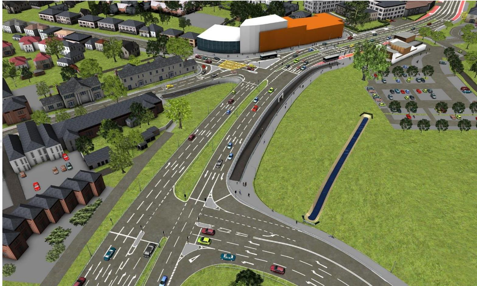
Two new T-junctions created – one linking Essex Yeomanry Way and Chelmer Road, and the other linking Essex Yeomanry Way/Parkway and Van Diemens Road/Baddow Road. Traffic signals would be used to control traffic flow at the junctions.
