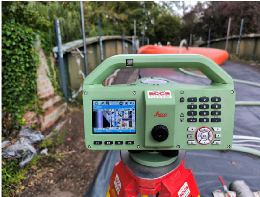
Figure 5 Leica LS15 Precision optical level positioned behind the south abutment (shown targeting the farthest measurement point on the west girder)
