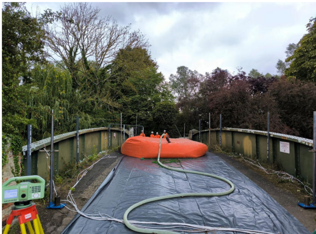
Figure 1 - Load testing of Boxted Bridge (load shown is approaching 12.2 tonnes)
