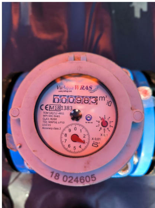
Figure 4 Calibrated analogue water flow meter (reading shows 983.931 \text{ m}^3 )
