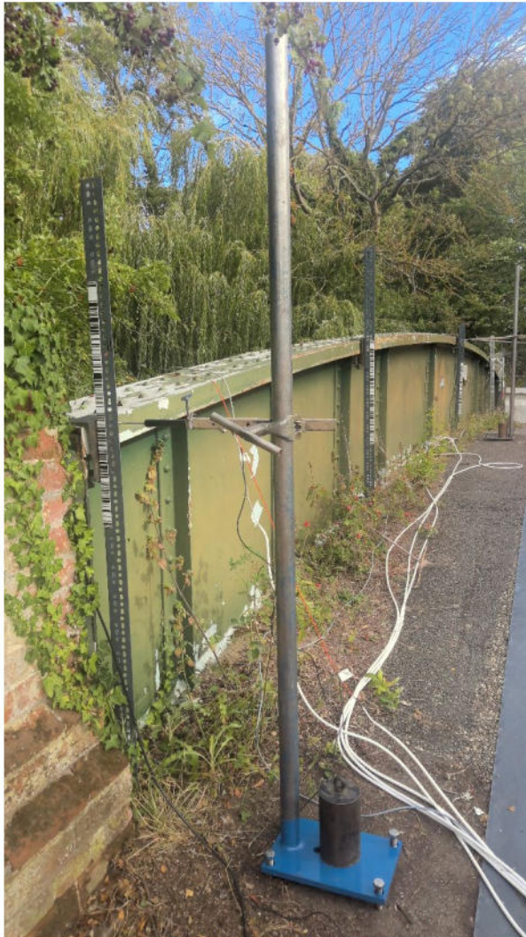
Figure 7 Displacement gauge mounted to weighted steel post
