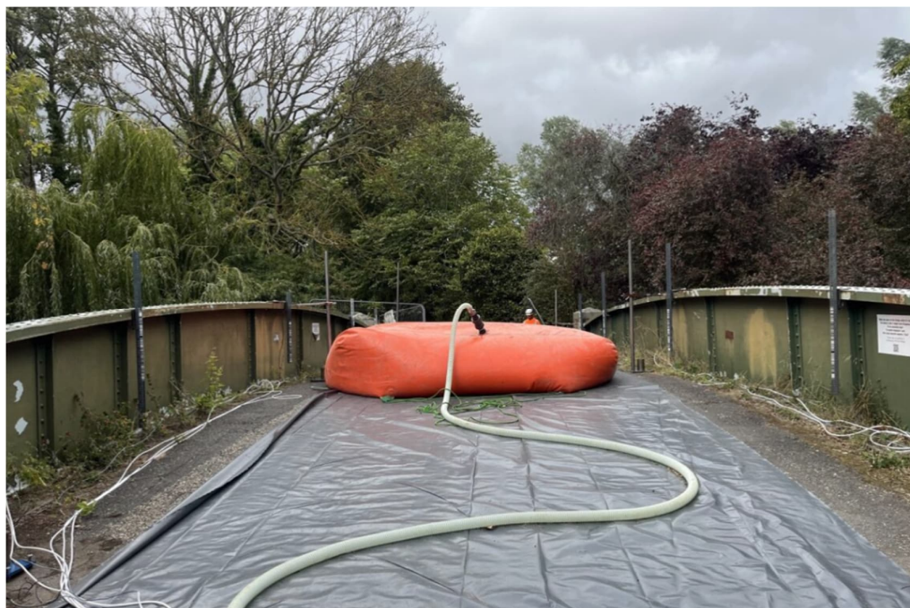
Figure 1. Botted Bridge Load Test
