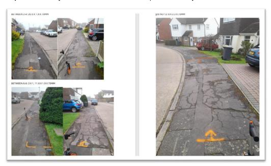
**Example 2** - Footways with kerbs. Two footway patches of approximately 12 metres in length including kerb replacement and one arterial gully replacement. Estimated completion is 3 days.
