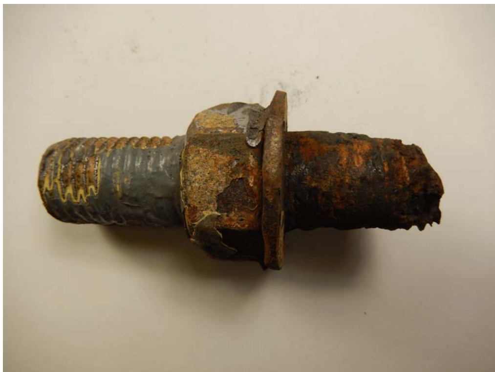
Photograph 2 End of failed holding down bolt, sample MY 775, showing coated threads above the mounting plate and corroded threads below the level of the mounting flange, in an area that would be surrounded by grout.
