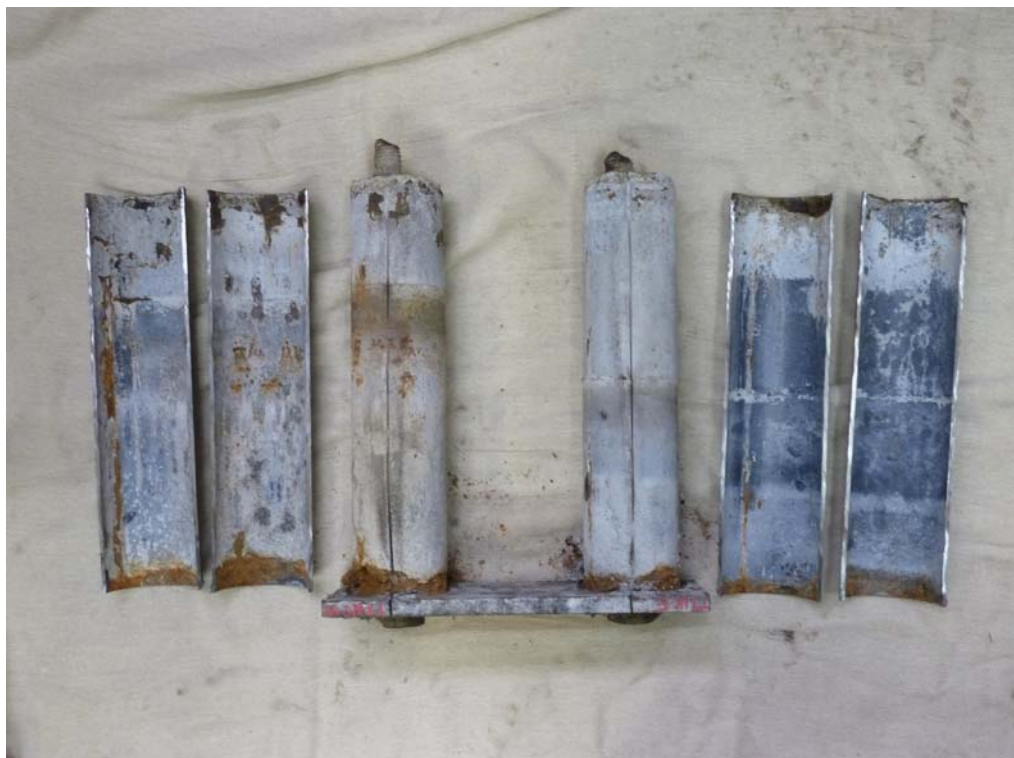
Photograph 4 Metal tubes removed exposing grout fill. Grout in tubes appears to have been filled in two goes, with an interface between the separate fill materials.
