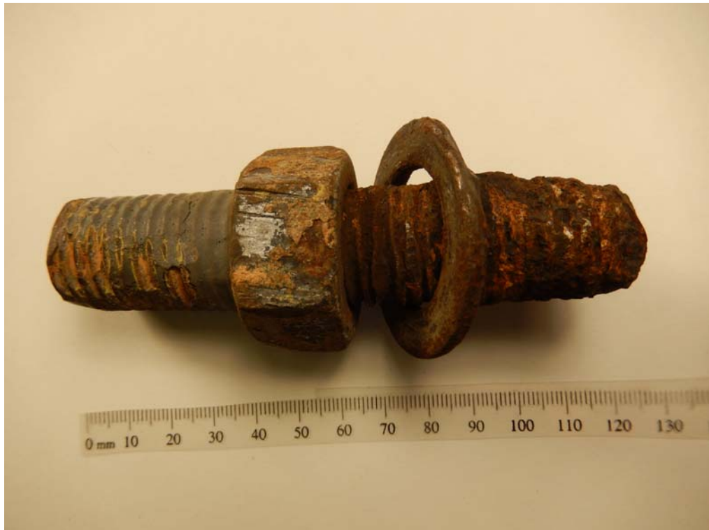
Photograph 1 End of failed holding down bolt, sample MY 774, showing coated threads above the mounting plate and corroded threads below the level of the mounting flange, in an area that would be surrounded by grout.
