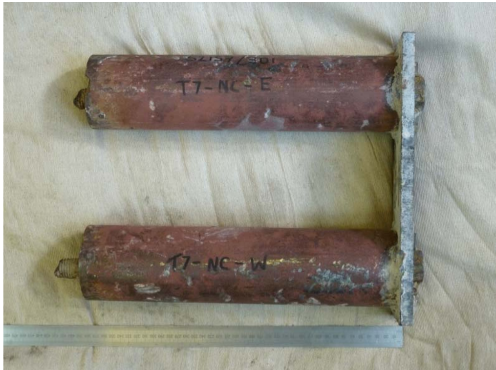
Photograph 3 Metal tube filled with grout surrounding the holding down bolts. Bolts had been inserted from the underside, such that the threads were uppermost to engage with flange under column.
