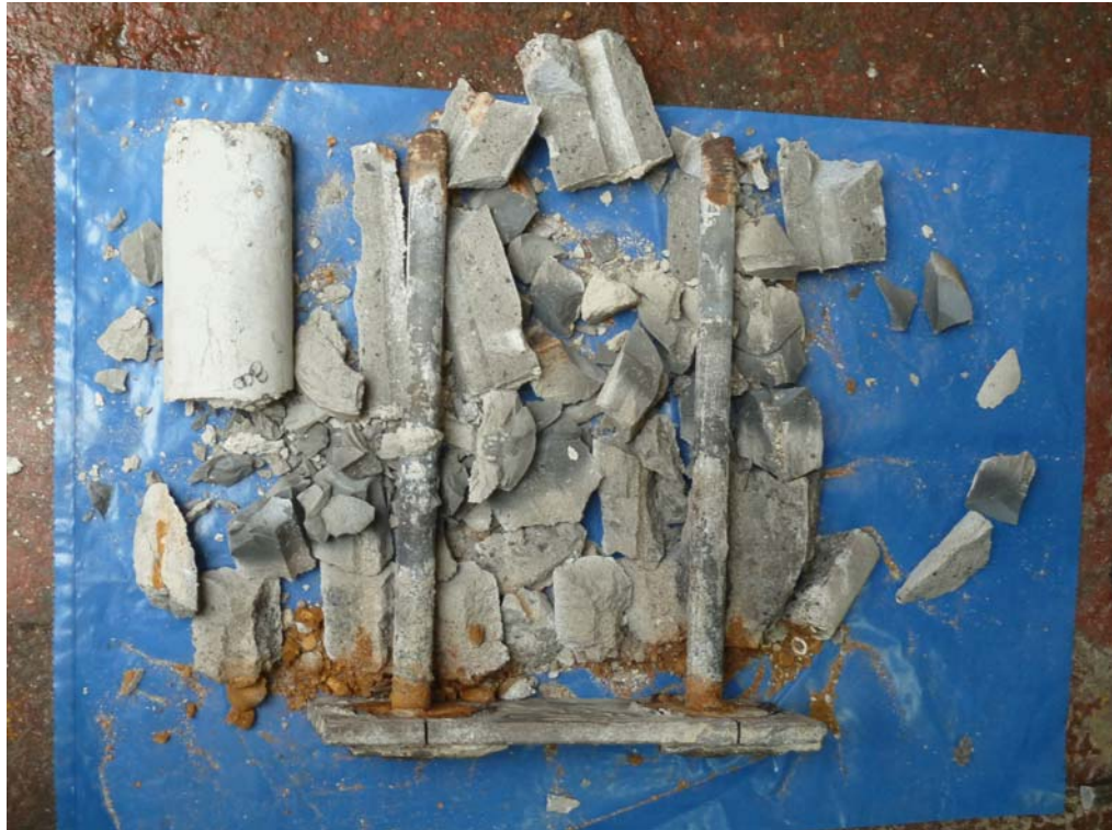
Photograph 5 Grout removed to expose shanks of holding down bolt. There was no evidence of corrosion or section loss of the bolts over the length within the grout tubes.
