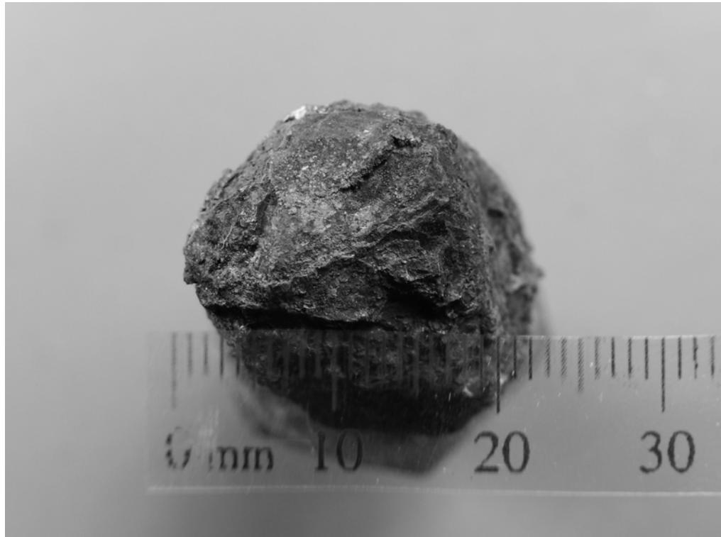
Photograph 7 End of sample MY 774 showing complete loss of section due to to corrosion. There was no evidence of fracture on this sample.
