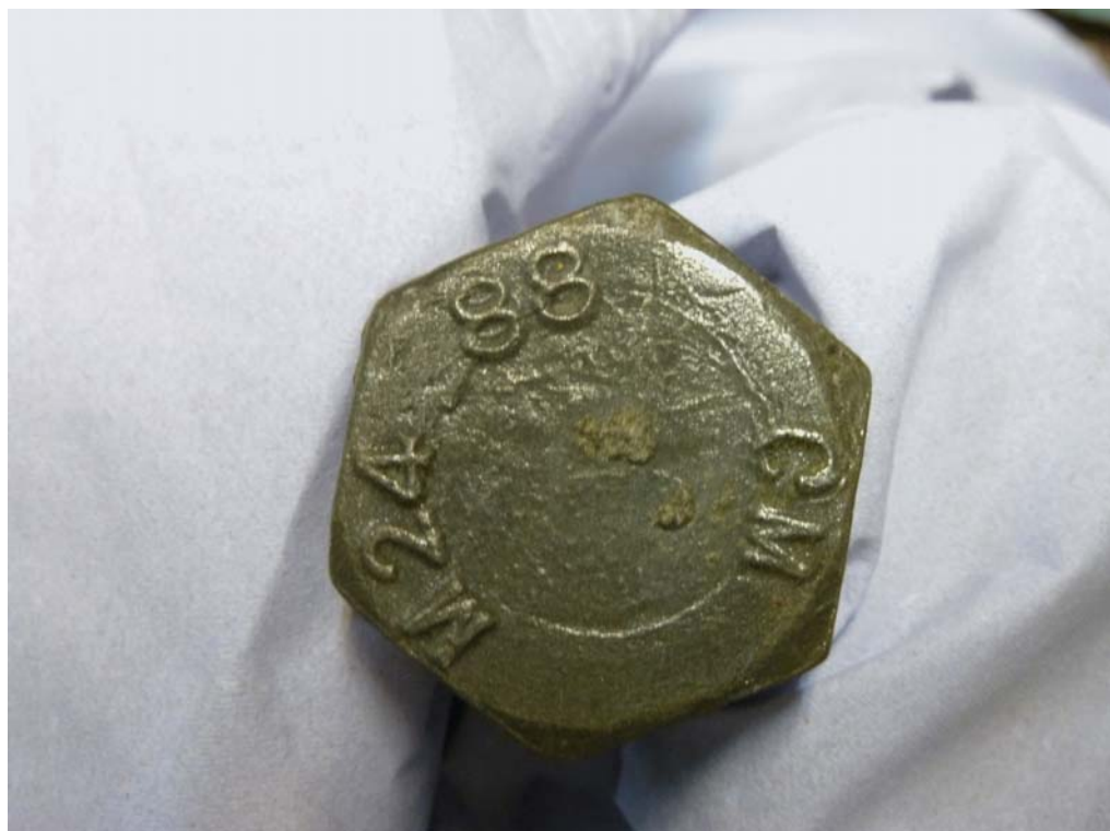
Photograph 6 Head of bolt showing size, 'M24', grade '8.8', and manufacturer's mark, 'CM'.
