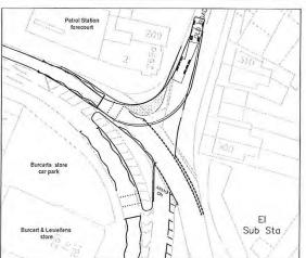
INSET 1: FTA 1998 design HGV left turn into Old Rd with new footway build out (Scale 1:500) ion of Ordnance Survey on behalf of the
