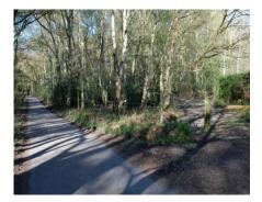
The provision of some form of levelling and surfacing, commonly tarmac (blacktop), for urban footpaths and an unbound surface such as Breedon gravel or road planings, sometimes capped with granite dust, for byways or bridleways in more rural settings.
