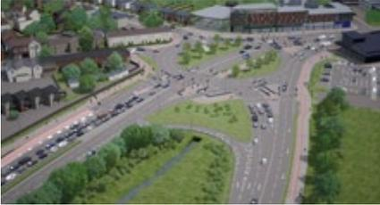
A Hamburger Roundabout allows the main road to pass through the middle while other routes go around.
