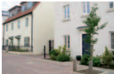
Left: Shared surface street using block paving with parking space defined using a different size and colour block. Upton, Northamptonshire
