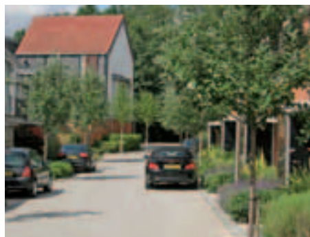
Shared surface at Newhall Harlow using natural bound gravel with granite setts
